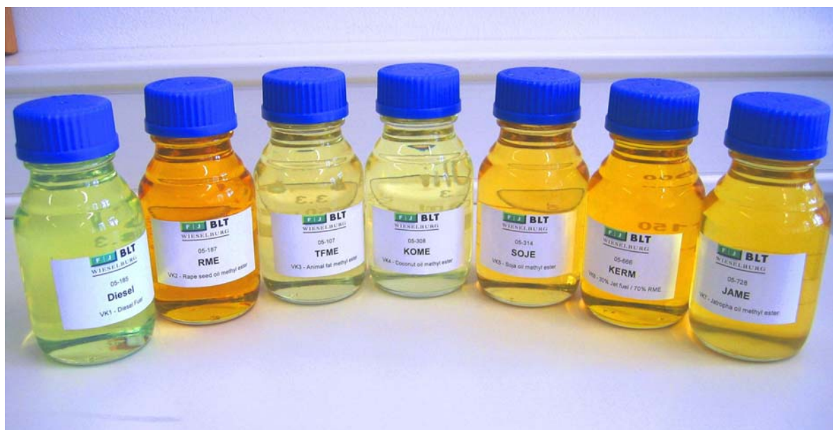
Figure 5: Test fuels for the endurance tests
