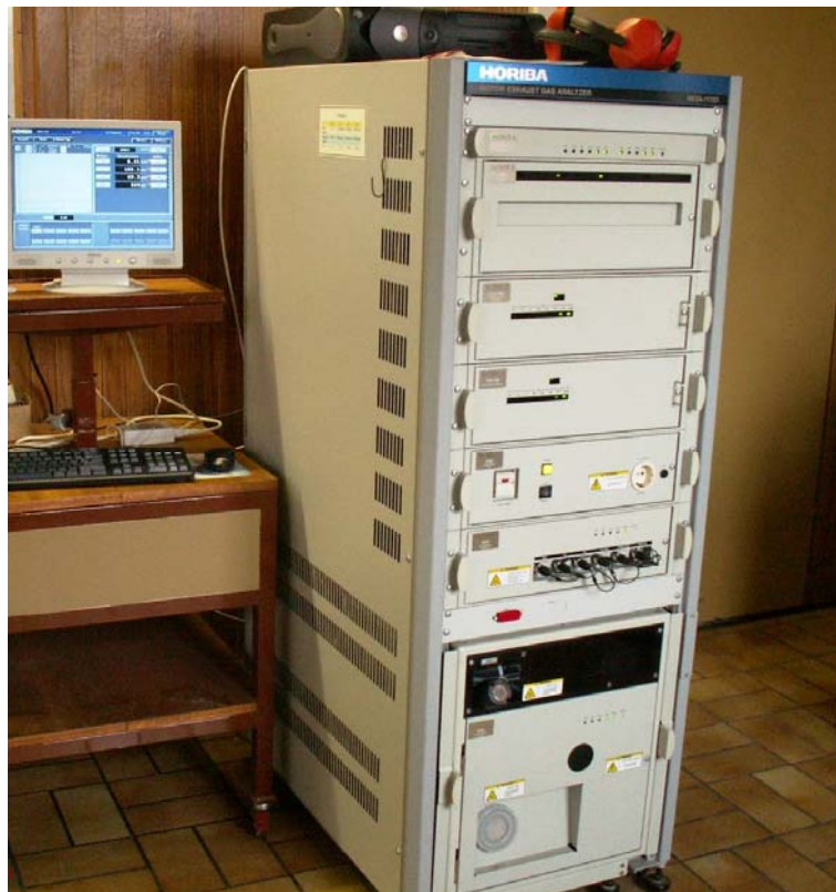
Figure 9: Emission test bench Horiba MEXA 7170 D
