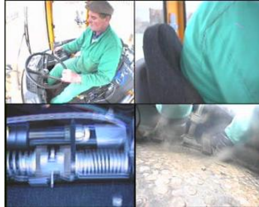
Figure 3.1.7 The four views recorded in the cab: hands location, contact area back/backrest, fore-and-aft suspension, feet position
