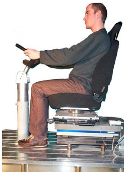
Fig. 3.3.2 Seat mounted on a shaker to measure the apparent mass of a seated subject.
