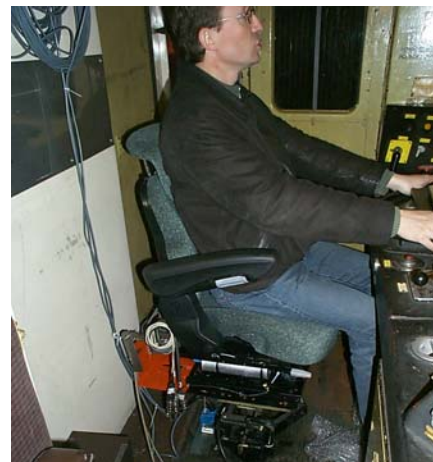
Figure 3.1.11 Vibration behaviour tests on the SNCF locomotive
